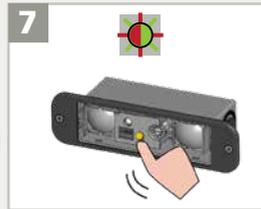
Push the push button shortly to launch an automatic setup. The LED will flash RED-GREEN.
