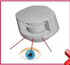
Do not stare into the visible red laser beams.
