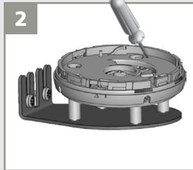
Position the mounting bracket and fasten the 4 screws firmly in order to avoid vibrations.
