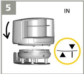
Position the housing on the mounting base.
