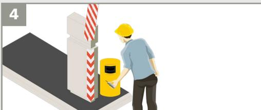
4 To finish, lock the sensor position by using a PH1 screwdriver.
