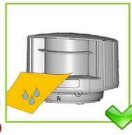
Clean the laser window with compressed air. If needed, wipe only with a soft, clean and damp microfiber cloth.
