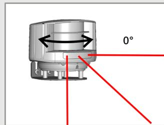
Turn the sensor slightly on its axis to adjust the lateral angle of the sensor to place the 0° laser spot on the reference.
