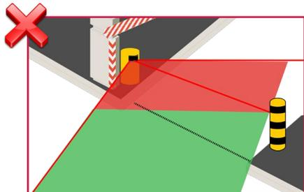
Do not position the detection field as shown.
