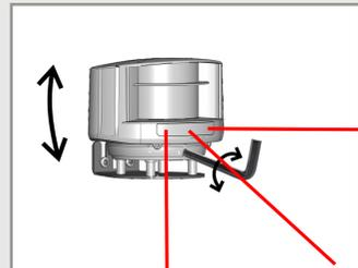
Adjust the tilt angle of the detection field with the hex key if necessary.
