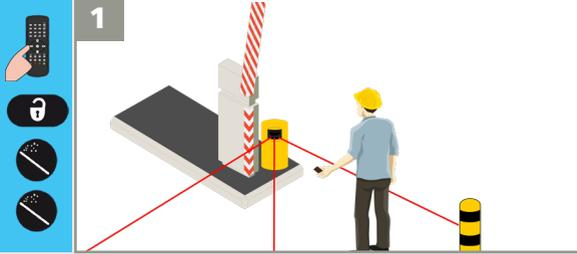
1 Activate the visible laser beams by remote control to position the sensor correctly.
