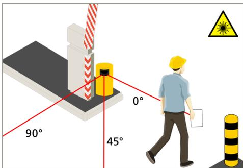
The sensor and detection field position are very important for the good functioning of the barrier.
