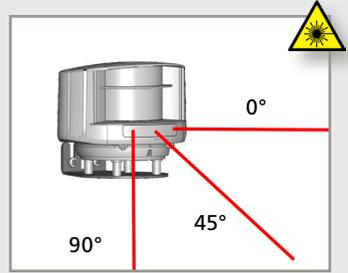
To turn them off, use the same sequence. After 15 min. the beams switch off automatically.
